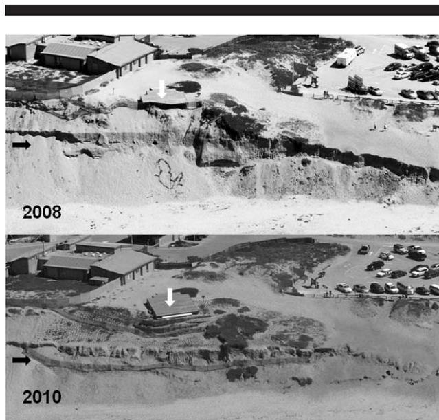
Figure 5. Aerial photographs of the Marina launch ramp at Marina State Beach captured in 2008 and 2010. Shoreline recession was measured at up to 8 m in this area. [Photos copyright (c) 2010, Adelman and Adelman (2010), Kenneth and Gabrielle Adelman, California Coastal Records Project, www.californiacoastline.org.] Resistant horizontal band in sealiff is a paleosol within the Quaternary Aromas Red Sandstone depicted with the horizontal black arrows.
